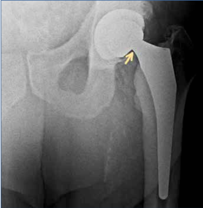
Figure 3. Anteroposterior radiograph, seven months prior to the fall, showing eccentric positioning of the trunnion in the femoral head, suggesting significant wear without complete fracture of the trunnion (yellow arrow). This rare radiographic finding is essential to recognize as impending trunnion failure.
