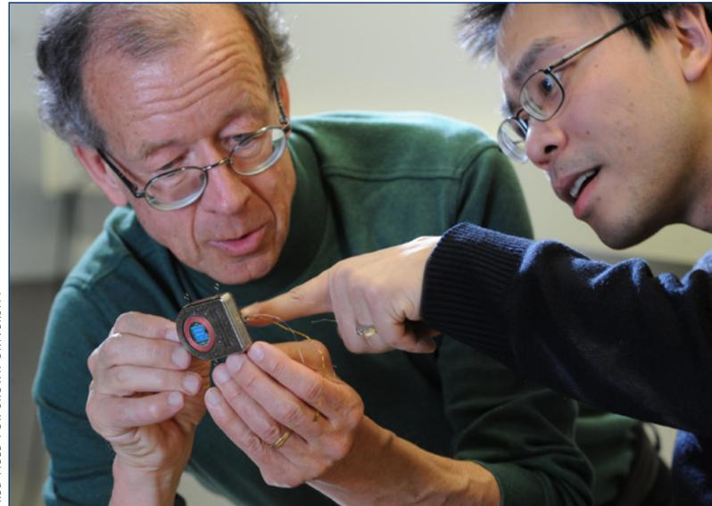
In a significant advance for brain-machine interfaces, engineers in the Brown Institute for Brain Science have developed a novel wireless, broadband, rechargeable, fully implantable brain sensor that has performed well in animal models. Here engineers Arto Nurmikko and Ming Yin examine their prototype device.
