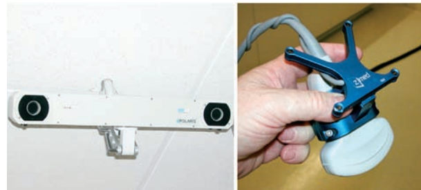
Figure 4 Image guidance using 3D ultrasound. The ceiling mounted stereoscopic digital cameras locate the ultrasound images by tracking the embedded reflectors in the handheld transducer.
