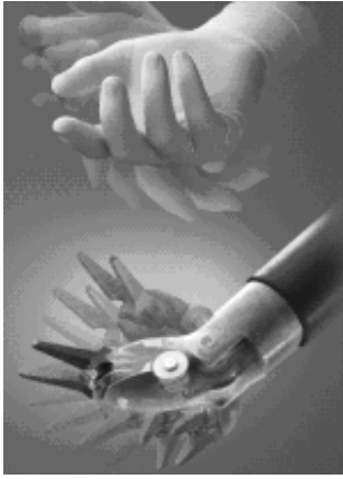
Image 1: Endowrist articulated instruments with 7 degrees of freedom. 2005 Intuitive Surgical, Inc. [Image courtesy of intuitivesurgical.com 2009]
